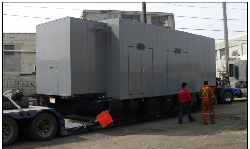
From top: Weather-Protective Sub Base Tank/Enclosure Package. Sound-Attenuated Enclosure package ships from Tramont's manufacturing and packaging facility.
