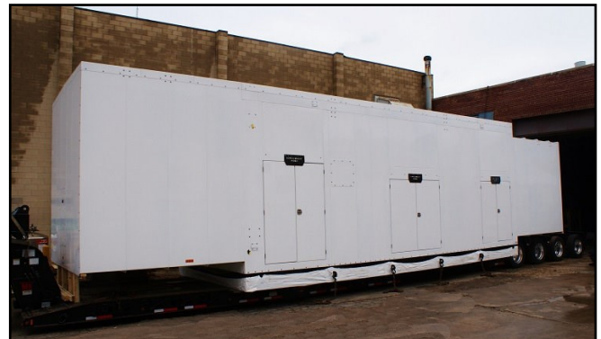
Right: 50-foot-long Sound-Attenuated Enclosure Package mounted on lifting base departs Tramont.
