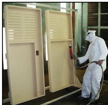
Left: All Tramont Enclosures receive a durable powder coat finish. Right: Enclosure powder coated in Oxide Red, one of 13 standard color selections.
