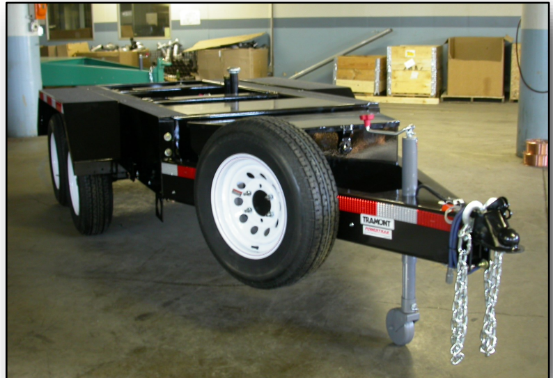
Tramont POWERTRAK trailer before mounting of genset. This dual axle trailer includes an optional spare tire.
