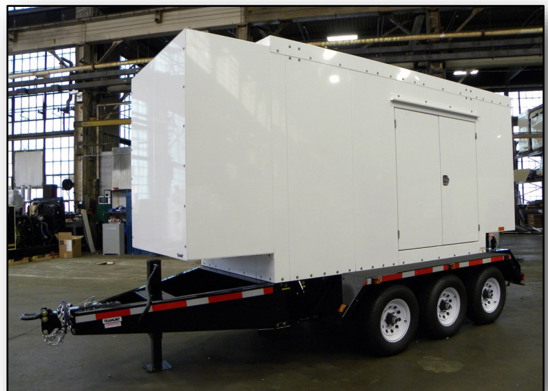
Enclosure and generator mounted on tri-axle trailer.
