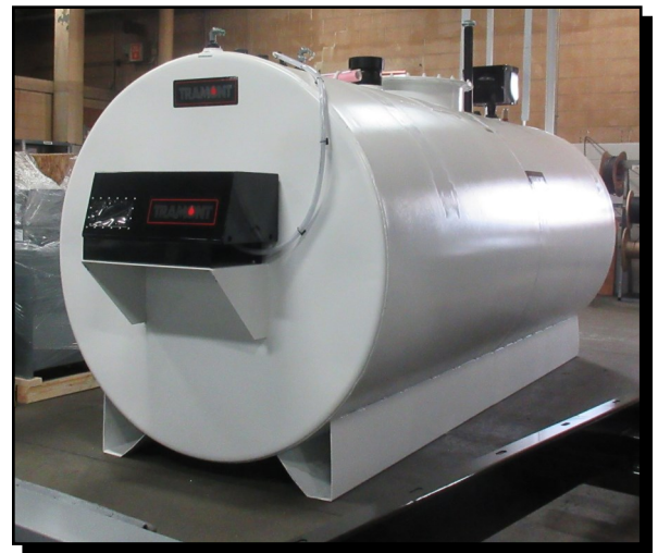
UL-142 Cylindrical Main Tank configured as a day tank. The pump, motor and controller are installed under the optional weatherproof cover visible on the end of the tank. "Saddle" for mounting tank to pad is also visible in this view.
